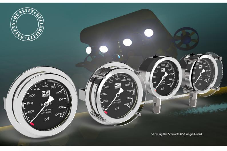
The **Stewarts-USA** range of compensated subsea pressure gauges have a 100% filled case that has a special compensation device, allowing the internals of the case to be pressurized equal to the external ambient pressure as the gauge is submerged to depth. The benefit of this method is that as the internal and external pressure remain in balance, there is no need for a pressure proof case, allowing our 8000 series subsea compensated gauges to work at your deepest depth applications.
