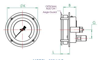
MODEL - 8024/AG Flush Mounted - Clamp Fixing with Aegis-Guard
